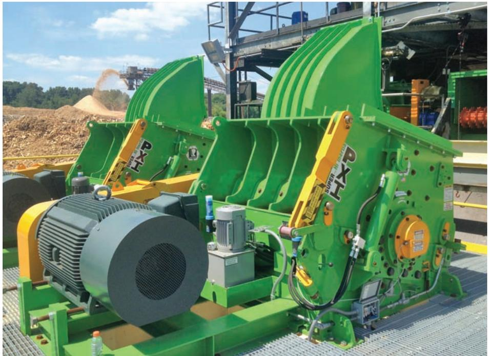
**TWIN HOGS:** *The Twin Rawlings 36x60 Vertical hogs are designed to handle all kinds of hard-to-grind materials including stringy cedar bark, green spruce bark, all kinds of mill wood waste, demolition debris, butt ends and railroad ties. The vertical hogs are shown here processing white wood chip overs at a paper mill.*
