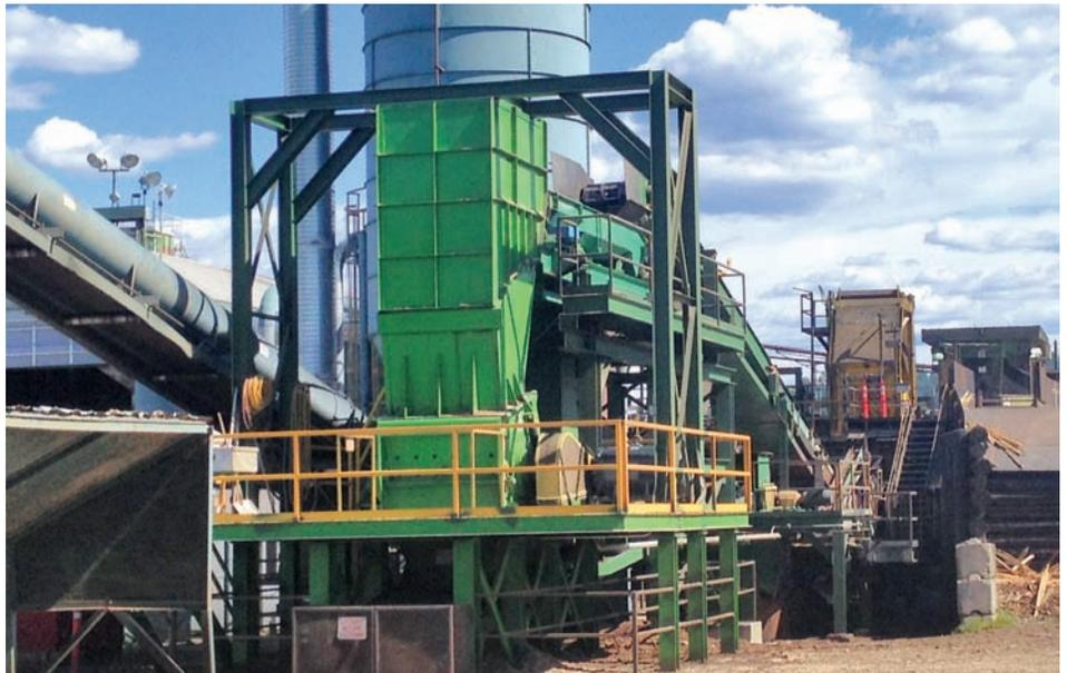
**36x60 VERTICAL HOG:** A 36x60 Rawlings Vertical Hog processes wood waste at a plywood mill. Rawlings hogs were developed from rock crusher technology and uses both shear and impact to reduce material.
